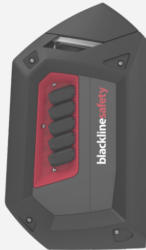
Four-channel pump module installed
